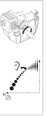
needle is adjusted correctly when the machine 'splatters' a little . If the machine smokes heavily at the same time as it 'splatters' heavily the adjustment is too rich.
